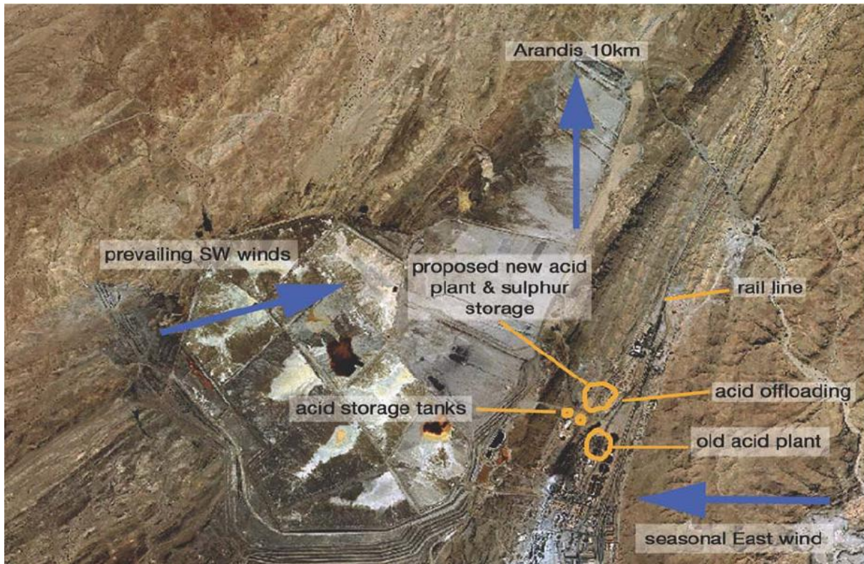
Figure 3-1 Overlain on an aerial photograph, the proposed location of the new RU acid plant relative to the existing acid plants and other related sulphuric acid producing infrastructure (source: RU public participation material, 2007)
