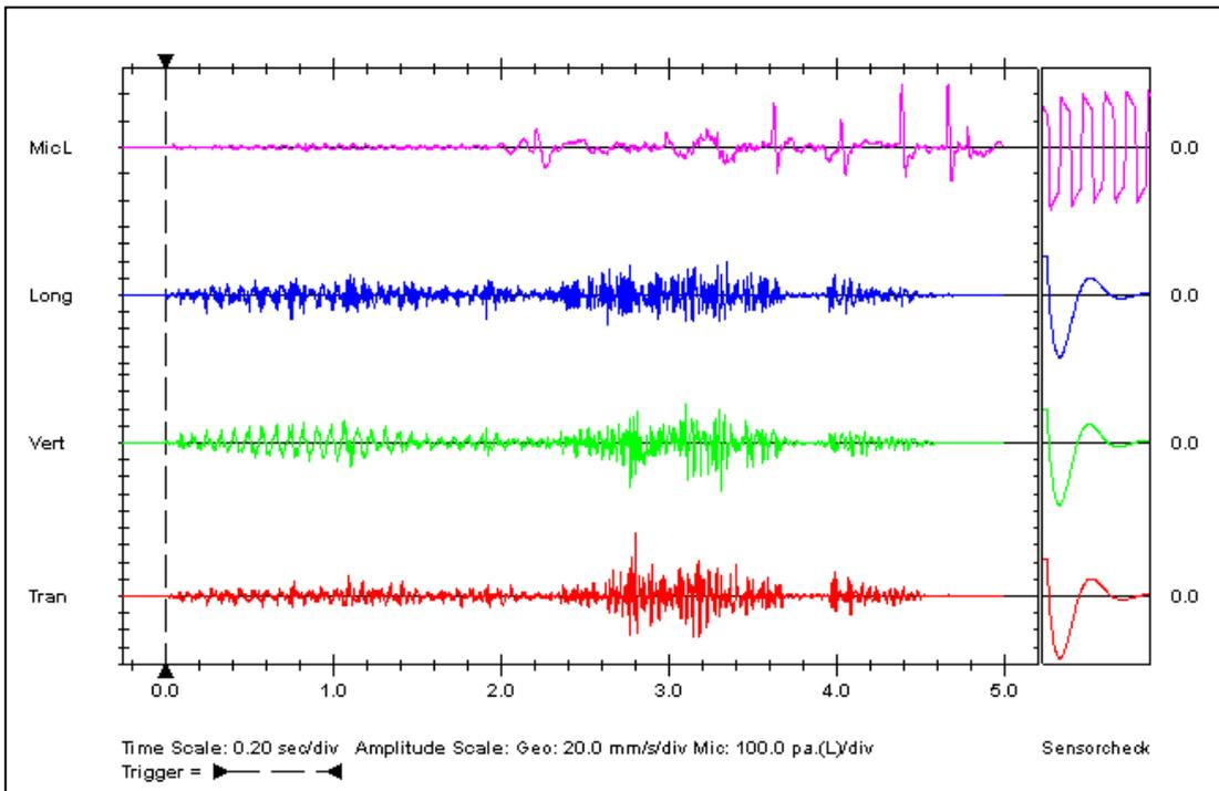
Trace shows proper ground vibration and air blast as recorded from the blast.
