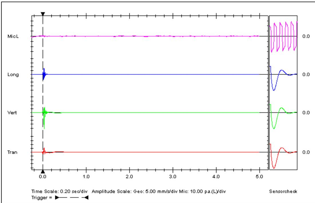
Trace shows a false trigger on the ground vibration. It is suspected that something has dropped onto or moved the sensors.
