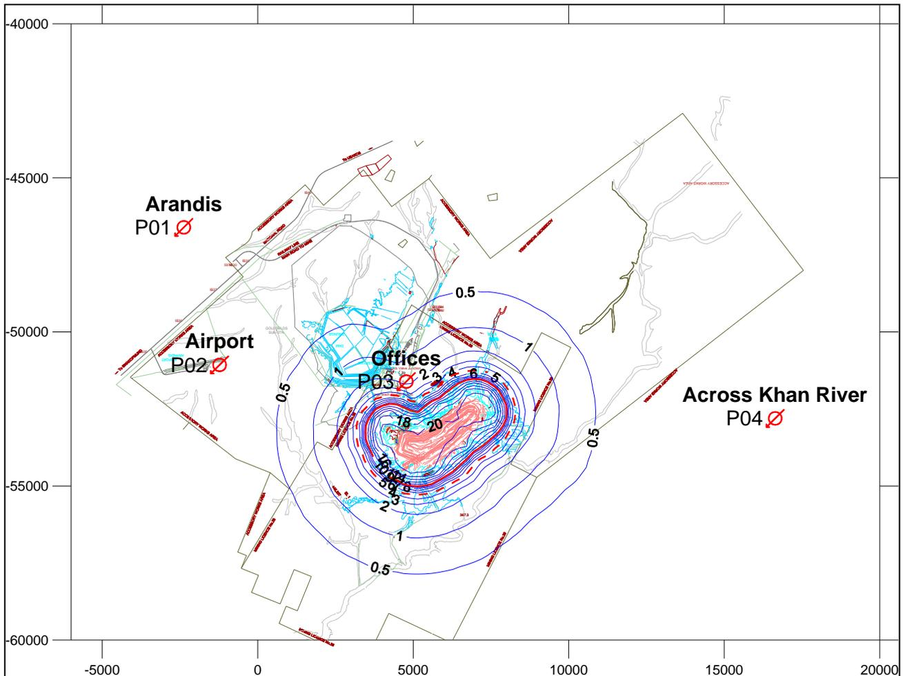
Note: Red dotted line is the 10mm/s level and Solid Red line is the 5mm/s level.
