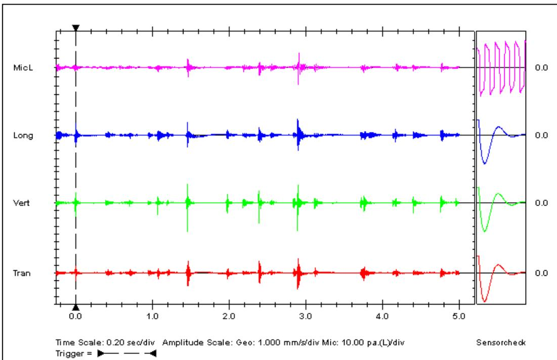
Trace shows false triggers on all the sensors. Note that all activities occur at the same time. This could have been movement or bumping against the box in which the seismograph is housed.
