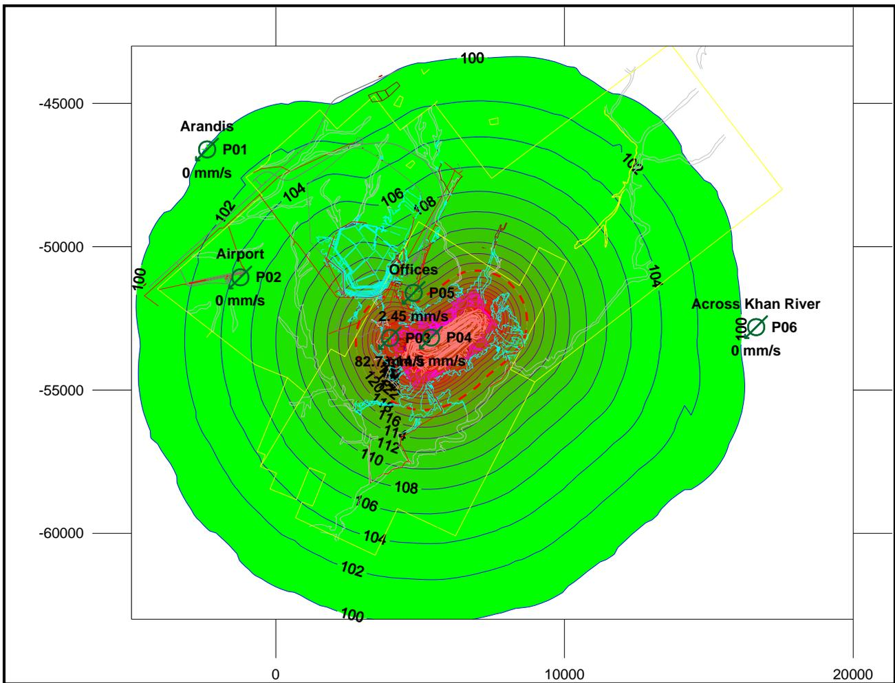
Note: Red dotted line is the 10mm/s level and Solid Red line is the 5mm/s level.
