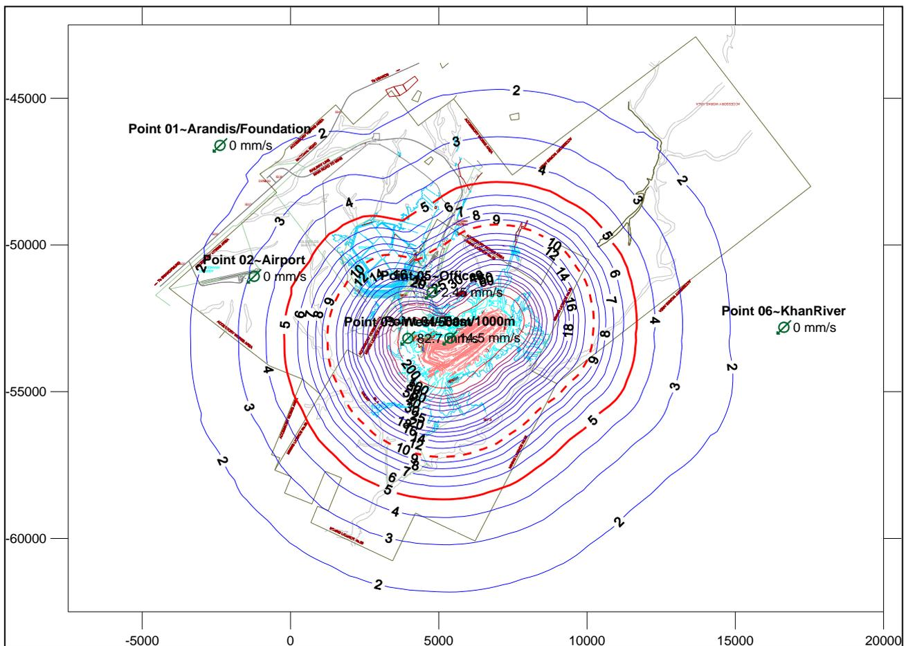
Note: Red dotted line is the 10mm/s level and Solid Red line is the 5mm/s level.
