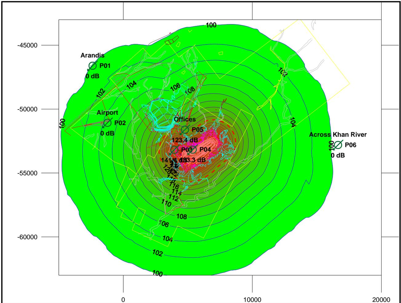
Considering the actual and predicted levels for ground vibration, a further aspect that needs to be addressed is at which stage the minimum limit levels will be reached. The maximum charge mass required producing at least 5mm/s ground vibration was calculated and is shown in the Figure 28 below.
