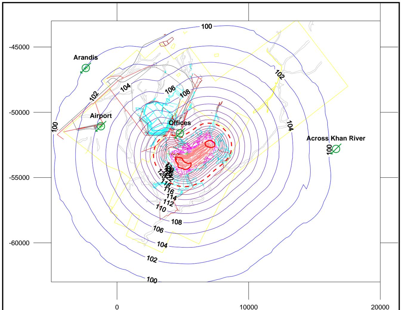
Note: Red dotted line is the 120dB level and Solid Red line is the 134dB level.
