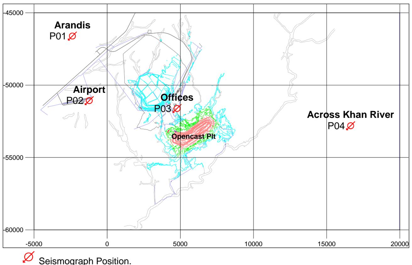
The four monitor positions will cover the private installations, i.e. the Arandis airport, Arandis town and the farmers across the Kahn river. The monitor at the office is a control point and can be used to verify results obtained at any of the other positions. This monitor is likely to be the only one triggering. Blasting in various areas of the pit will yield different results. The office monitor will help build a database for assessing the influence from blasts at different locations.
