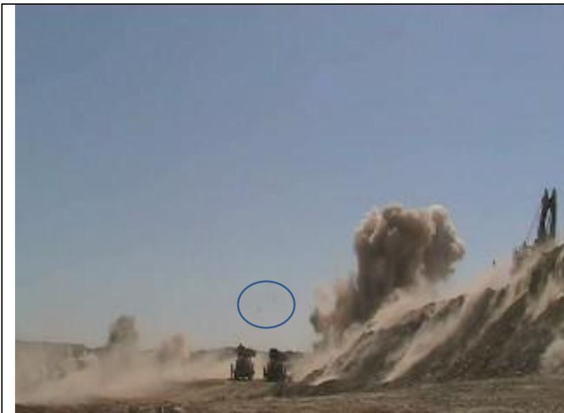
Circles show pieces of rock elements that were propelled from the blast and on the downward trajectory.
