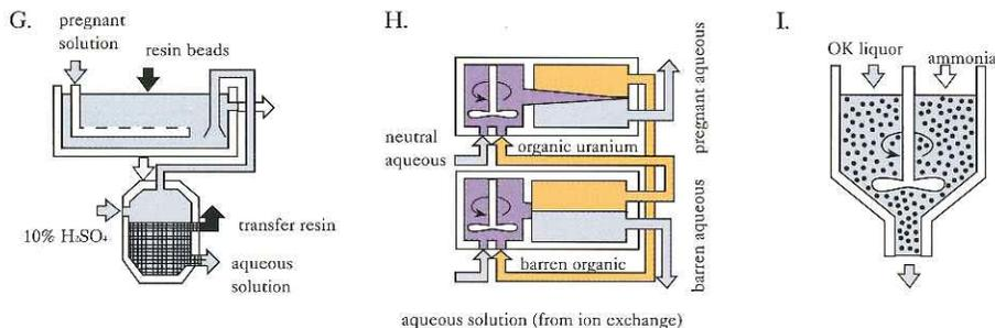
**G. CONTINUOUS ION EXCHANGE:** CIX(11) The clear pregnant solution now comes into contact with beads of specially-formulated resin. Uranium ions are absorbed onto the resin and are preferentially extracted from the solution. Beads are removed periodically to elution columns where a strong acid wash removes the uranium from the beads. The resulting eluate is a purified and more concentrated uranium solution.
