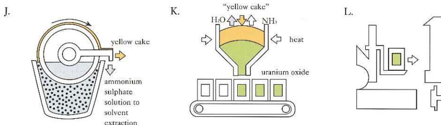
**J. FILTRATION** (13) The ammonium diuranate is recovered on rotating drum filters as yellow paste-'yellow cake'.
