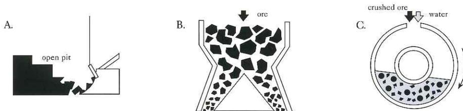
**A. MINING:** (1) The uranium ore at Rössing is recovered by drilling, blasting, loading and haulage. Due to erratic distribution of minerals in the ground, waste and ore are often mixed together. Radiometric scanners measure the radioactivity level of each truckload (1a). This determines whether the material is sent to the primary crushers (2) or to low-grade stockpile. Waste is transported to a separate dump.
