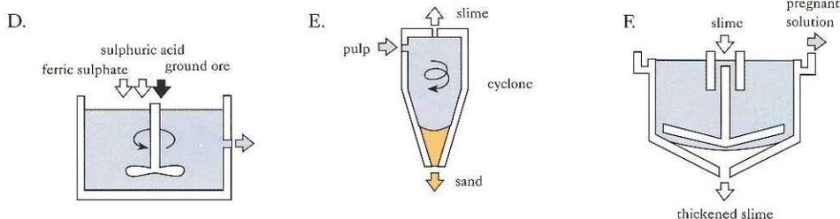
**D. LEACHING:** A combined leaching and oxidation process takes place in large mechanically agitated tanks (8). The uranium content of the pulped ore is oxidised by ferric sulphate and dissolved in a sulphuric acid solution. Sulphuric acid is produced through a pyrite-roasting process on site (14).
