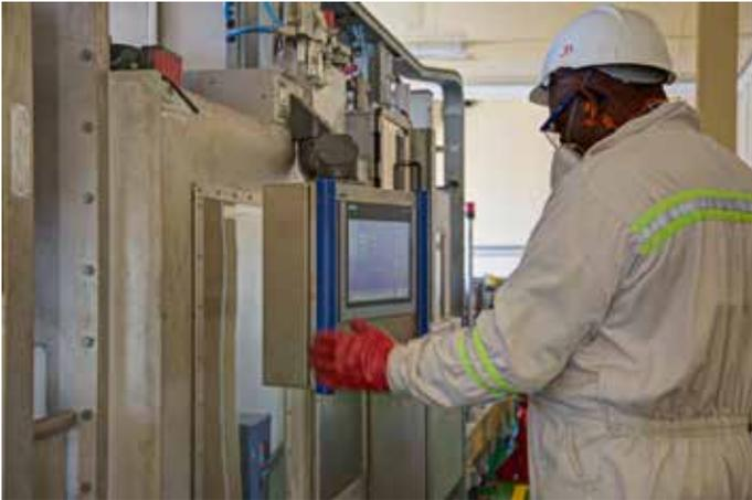
Unlike the old way of drumming where the dust could escape from the drum, the new method ensures that the filling compartment is totally enclosed whereby little to no dust escapes into the building.
