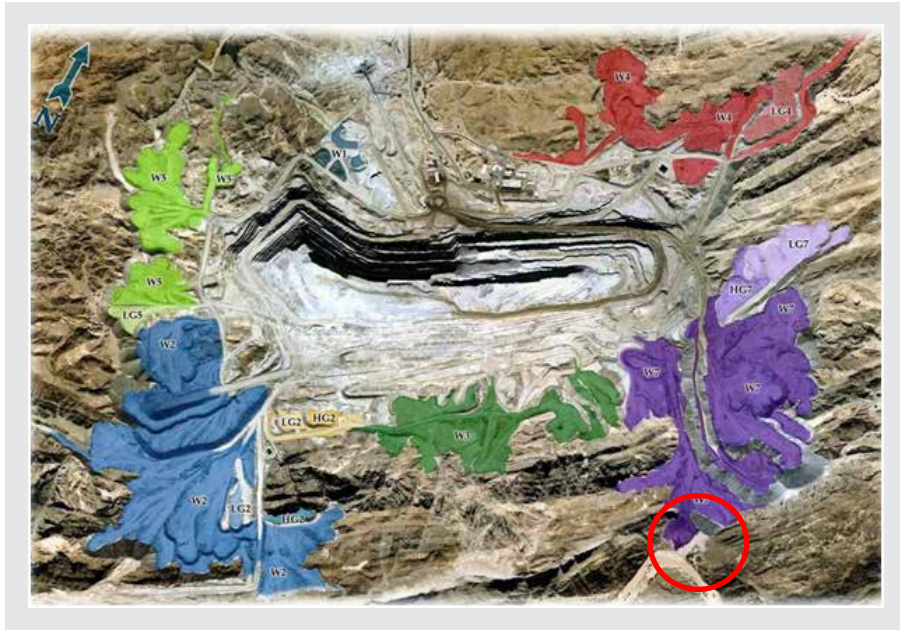
Figure 2: Location of waste rock dumps relative to the SJ Pit. The purple-coded Waste Rock Dump W7 borders the Dome Gorge. The Dome Gorge confluence with the Khan River is circled in red. (Source of map: Google Earth)
