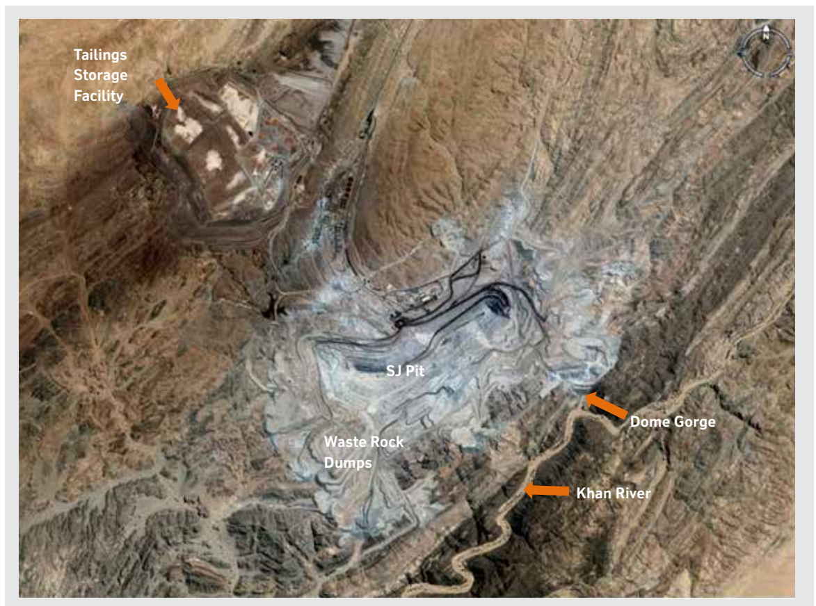
Figure 1: Rössing mine site including the SJ Pit, Waste Rock Dumps (lighter grey areas surrounding the pit) and Tailings Storage Facility. The Khan River is located to the south-east of the site. (Source of map: Google Earth)
